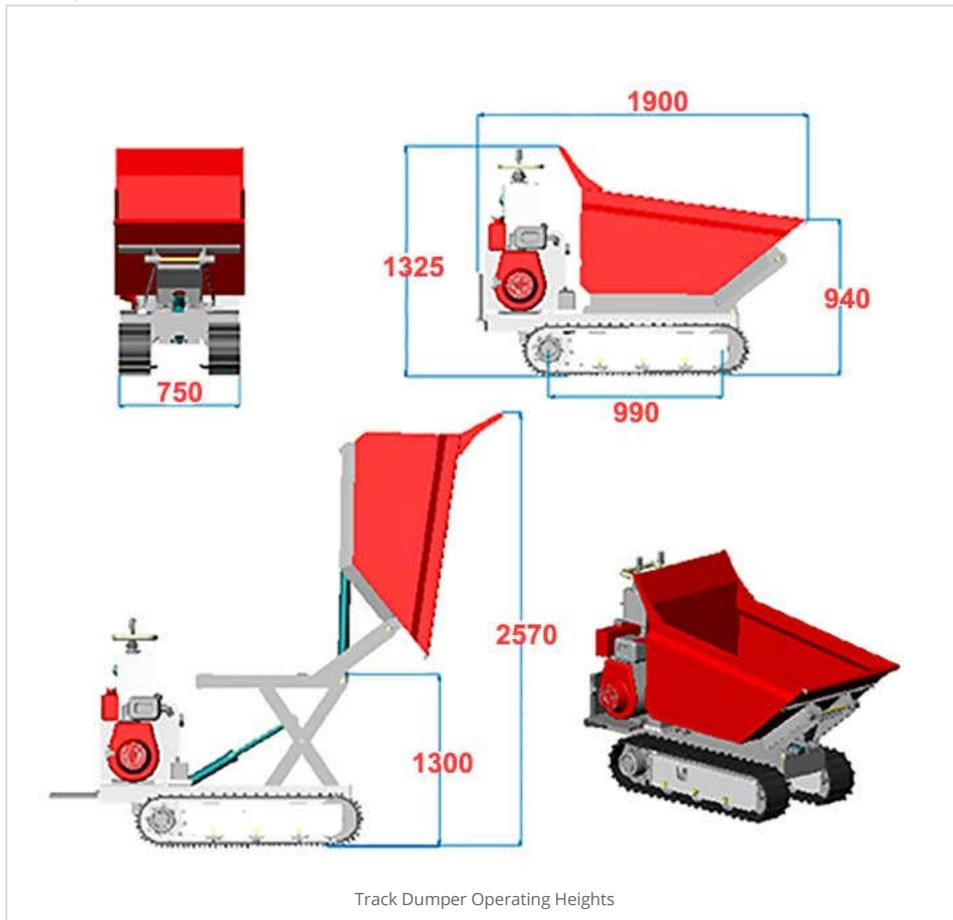
**Undercarriage:** Rubber tracks c/w planetary drive and negative brakes
